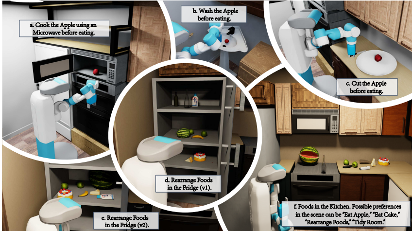
232 Figure 3: Example of preferences and their corresponding actions in PbP. Cooking using microwave (a), 233 washing in the sink (b), and cutting to halves (c) belong to the primitive action level preferences. For rearranging 234 objects, we present two option-level preferences of either grouping objects by their categories (d) or putting 235 them on the same layer of the fridge (e). For after-dinner activities, a user might want to first have fruits and do 236 some cleaning in the order shown in the sequence-level preference (f).
