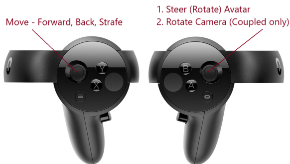
Figure 3: Oculus Touch control mappings.
