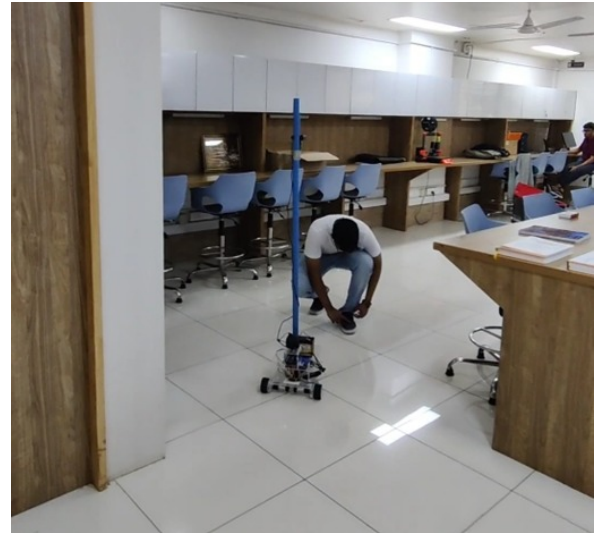
Fig. 6. The robot stopping as the patient stops following it.
