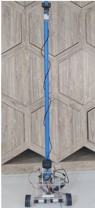
Fig. 2. The entire bot along with the camera and the pipe attached to it.
