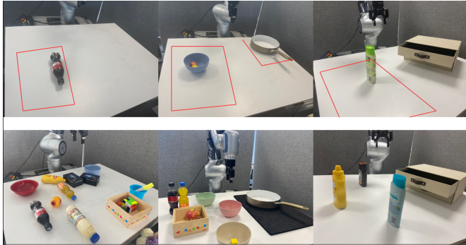
Fig. 3: Training scenes (top row) and cluttered test scenes (bottom row). The red lines indicate the position variations in collected demonstrations. From left to right, the tasks are bottle upright, bowl pour, and bottle in drawer.
