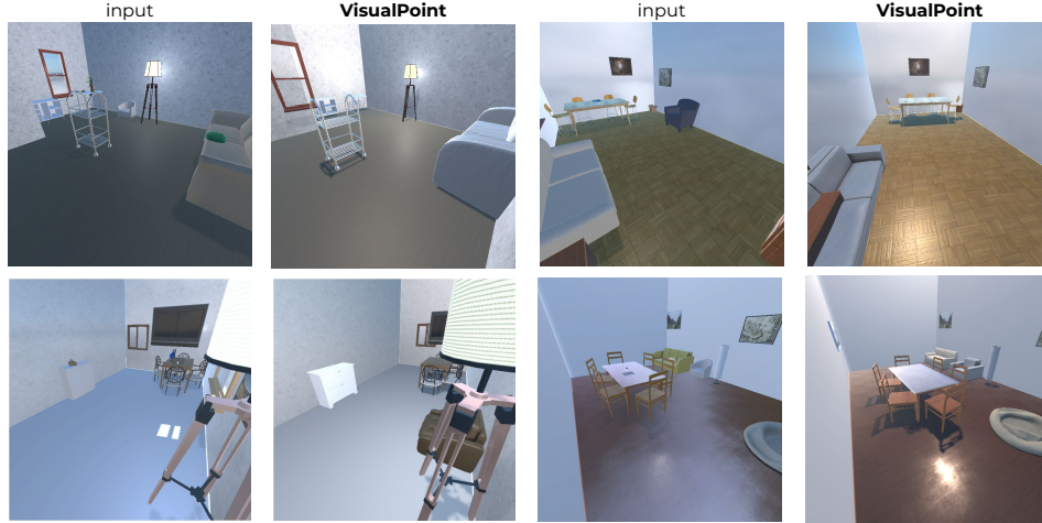
Figure 4: Qualitative results showing the input 2D image and the view rendered from the graphics program output of our VisualPoint strategy. VisualPoint is accurate at reconstructing the scene, although there are occasional errors in pose and object hallucination.
