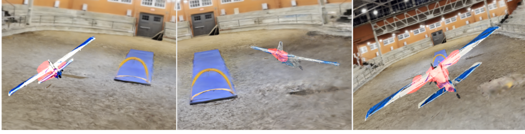
Figure 8: During training, we enable domain randomization in terms of leader gaussians’ color and scale to improve training and minimize the sim-to-real gap.
