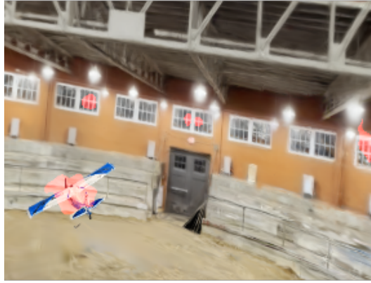
Figure 6: An example of failed detection where perception confuses leading aircraft with the background window using "Mask" approach in Section 5.2 that leads to downstream tracking error.
