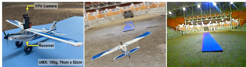
Figure 1: Left: Our ultra-light 150 g fixed-wing aircraft for indoor aerial research, equipped with a FPV camera and ROS-enabled autonomous control. Middle: Onboard view for leader-follower visual tracking using a digital camera. Right: Onboard view during autonomous landing using an analog camera.
