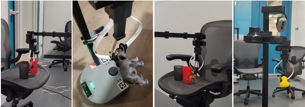
Figure 16: Grasping tests in various lab environments. To provide a strong baseline, we tuned the grasp policy to be highly reliable given the Stretch’s viewpoint, on a variety of objects.
