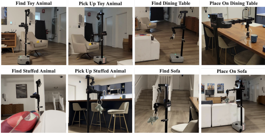
Figure 18: Real-world examples (also see Fig 2). Our system is able to find held-out objects in an unseen environment and navigate to receptacles in order to place them, all with no information about the world at all, other than the relevant classes. However, we see this performance is highly dependent on perception performance for now; many real-world examples also fail due to near-miss collisions.
