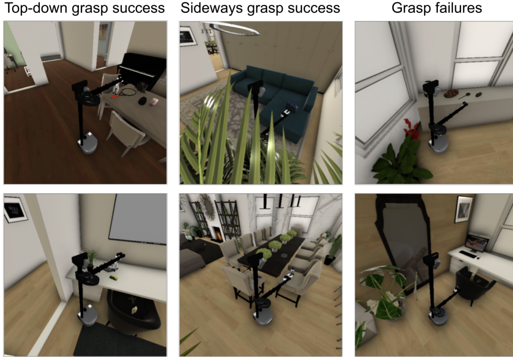
Figure 6: A few success and failure cases for our simple grasping policy under the new grasp success condition that requires the agent’s arm to reach near the object without colliding. The agent resorts to sideways grasps when the object can’t be reached via top-down grasp that bends the gripper. Most grasping failures are because of the collisions with the scene.
