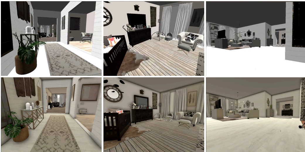
Figure 14: Here we present the improvements in scene visuals with Horizon-based Ambient Occlusion (HBAO) and expanded Physics-based Rendering (PBR) material support added to the Habitat renderer. The top row shows images from the default renderer whereas the bottom row shows the improved renderings.
