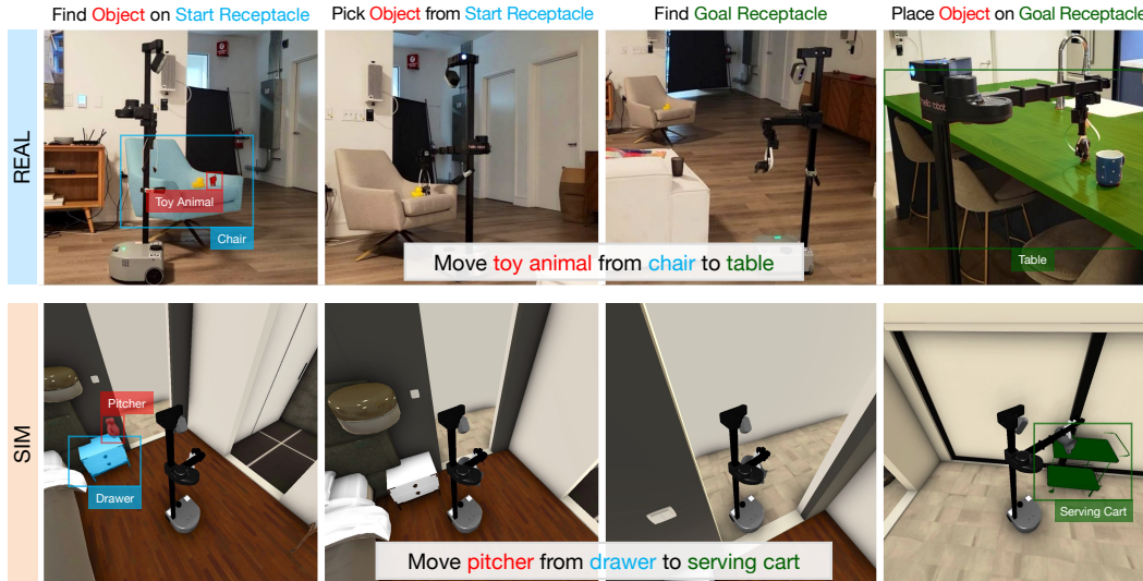
Figure 1: Open-Vocabulary Mobile Manipulation requires agents to search for a previously unseen object at a particular location, and move it to the correct receptacle.
