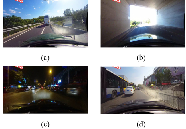
Figure 1: Some challenging scenarios for lane detection. (a) Demonstrates curved lanes, and our Angle Loss significantly improves the detection results in such scenarios. (b) Illustrates lanes under dazzle conditions, where lane detection heavily relies on global semantics. (c) Represents a no line scenario. (d) Depicts lanes are occupied by other vehicles, making lane detection exceptionally challenging.
