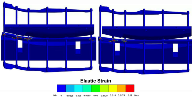
Fig. 6. Example of FEM simulation frames after preprocessing. Images are resized to 512 by 512 pixels after being cropped to focus on the relevant segments of the antenna configuration while removing unnecessary experimental references and backgrounds.
