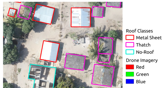
Figure C.8: Drone Imagery with RGB (Red, Green, and Blue channels) and annotations
