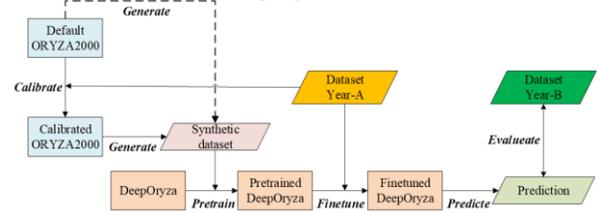
**Fig. 1** The framework for building and evaluating the DeepOryza model.
