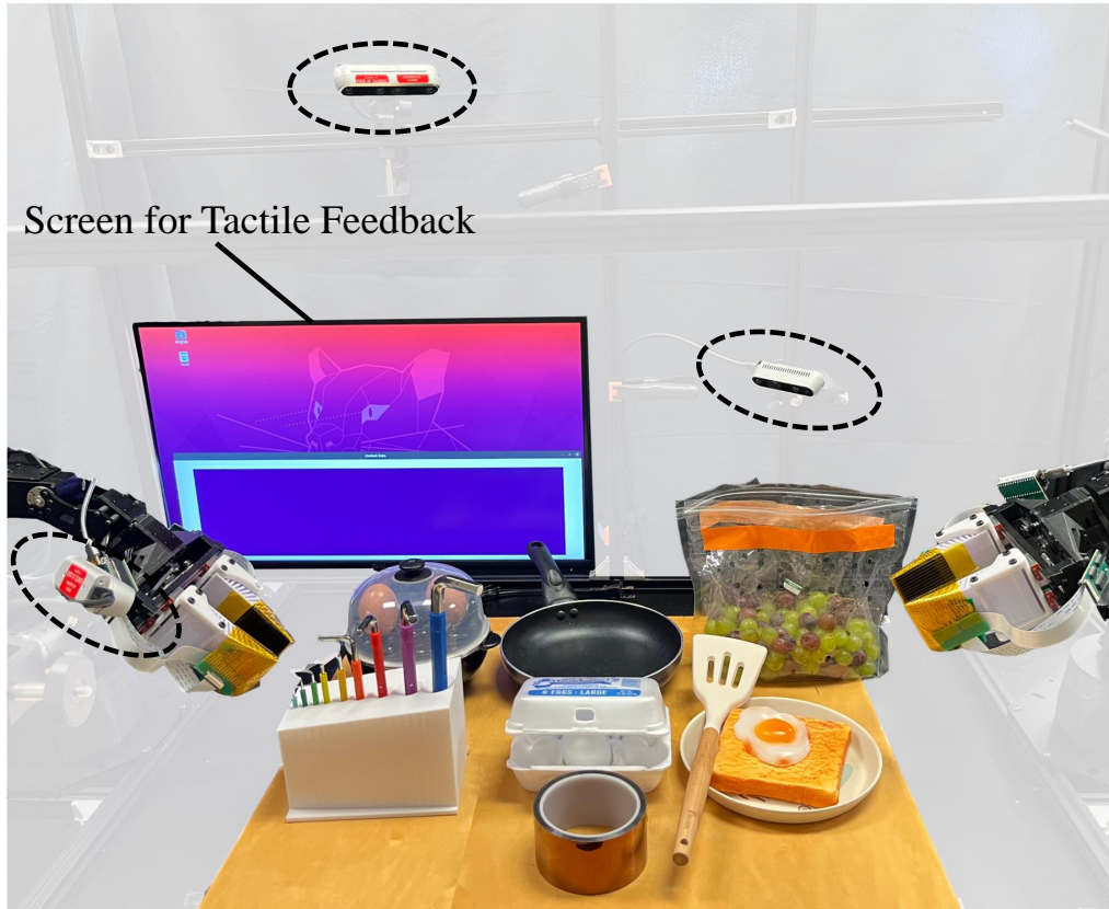
Figure 9: System Overview. We attach four tactile sensors to four robot fingers and install three Realsense cameras to cover the workspace. All the objects used for the task are shown in the workspace. Additionally, we install a background screen to display the tactile feedback.
