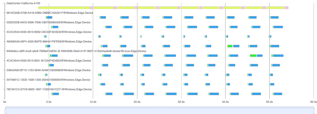
Figure 11: Real-world application demonstration. Yellow: aggregation server waiting time; pink: aggregation time; green: client training time; blue: client communication time.
