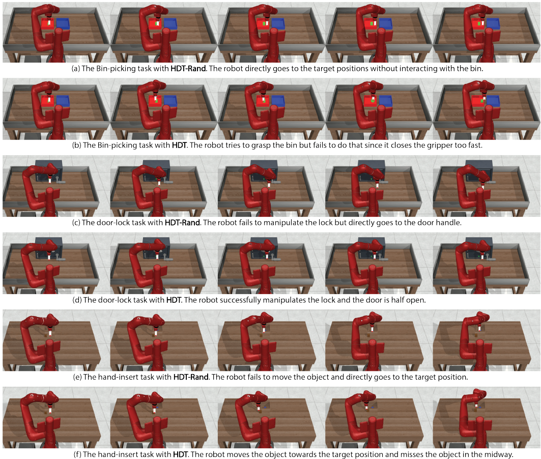
Figure 7: Environment Visualization. We provide key screenshots of three testing environment rollouts to compare the initialization of our proposed HDT and HDT-Rand, which randomly initialize the adapter layers.
