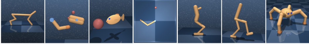
Figure 3: Domains from DeepMind Control Suite considered in our experiments - cheetah, finger, fish, reacher, hopper, quadruped and walker.
