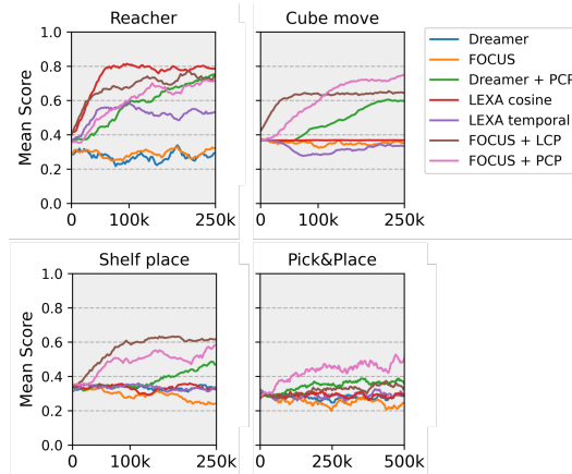
Figure 9: Offline training curves. Standard deviation is omitted for graphical reasons. Mean score refers to eq. 2 and is computed over 5 evaluation episodes, performed during the offline training. For each episode, a random goal is selected out of a pool of 10 manually engineered ones.
