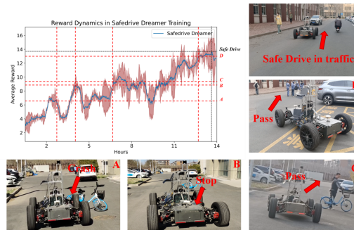
Figure 5. We present the curve showing the variation of the average reward of Safedreamer over time during training. On this curve, the actual reward at several specific time points is recorded. Concurrently, the vehicle states corresponding to these time points are displayed and illustrated through images A to D. For instance, during the process of generalizing the vehicle to real-world scenarios for learning, there was an increase in the reward curve, indicating an action to avoid obstacles. However, a collision still occurred, leading to a subsequent decrease in reward. This collision is represented on the reward curve by dashed line A, with the corresponding state time point documented.
