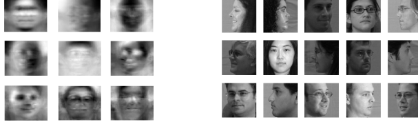
Figure 2: (a) The set of first 9 spectral components a.k.a. Eigen (Fisher) faces for 52,000 images from CMU Multi-PIE dataset. Linear combination of these components is able to reconstruct all 52,000 images with an average error less than 25%. (b) A subset of dataset with 15 images is found such that their span is as accurate as the span of the first 9 spectral components.
