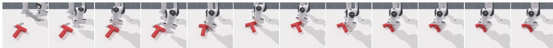
Figure 9: PushT Episode Visualization. The T-Block is pushed from sampled initial configuration to the goal area.
