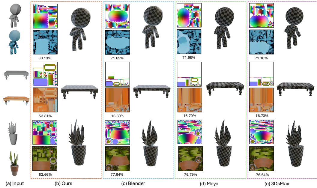
Figure 6: Qualitative Result on ArtUV-200K. (a) The input mesh and reference texture image. (b)-(e) Results of our method, along with Blender, Maya, and 3DsMax. For each method, the upper-left image shows the UV unwrapping visualized using normal directions, the lower-left image displays the texture map based on the reference texture, with the value below the texture map representing the UV utilization rate, and the right image presents the 3D model with a checkerboard texture.
