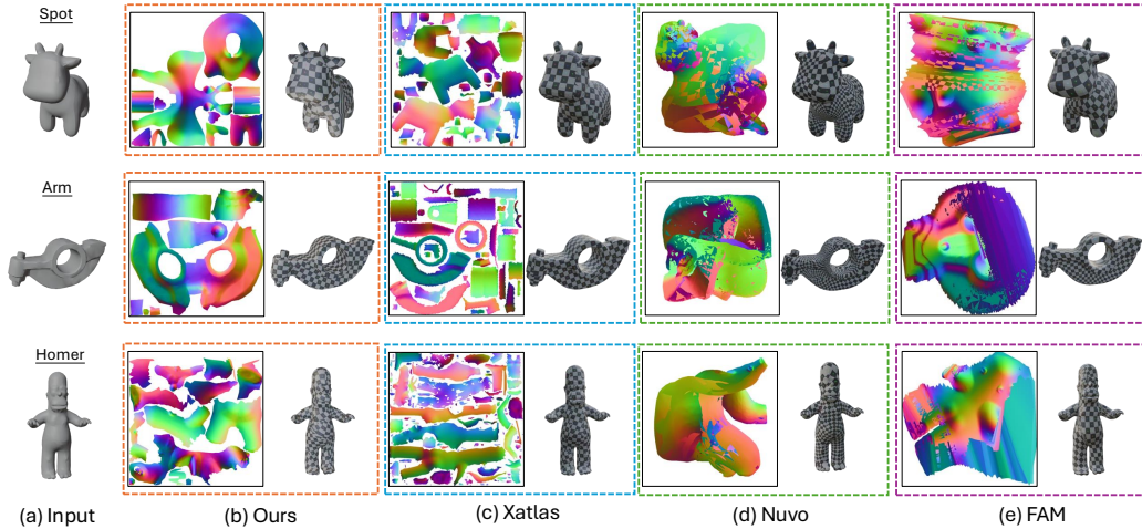
Figure 7: Qualitative Result on FAM benchmark(Spot, Arm, and Homer). (a) shows the input mesh from the FAM benchmark, while (b) to (e) present the UV unwrapping results for our method, XAtlas, Nuvo, and FAM, respectively. It is clear that our algorithm directly produces elegant and high-quality UV maps. In contrast, XAtlas results in overly fragmented and semantically weak UV maps, while Nuvo and FAM generate disordered and unusable UV maps.
