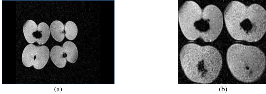
Figure 1: LF-MNR image preprocessing workflow: (a) simultaneous scanning of four apples; (b) 2 \times 2 merged apple region generated by the AppleNMR V1.0 module.
