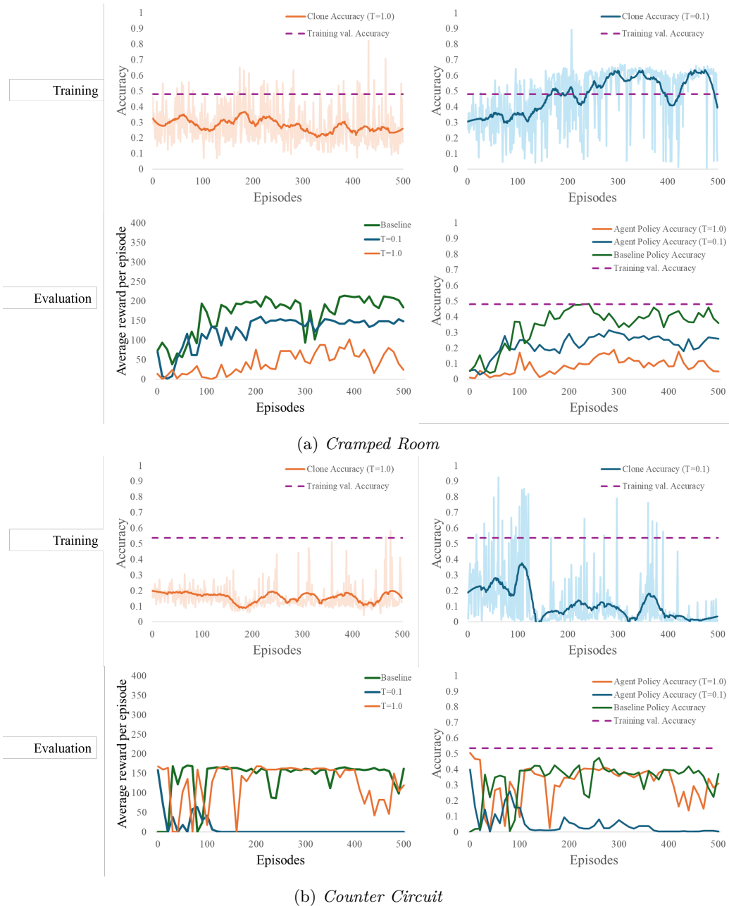
Figure 3: Top left: Clone accuracy at temperature=1.0. Top right: Clone accuracy at temperature=0.1. Bottom left: Evaluation results for each training checkpoint. Bottom right: Agent policy accuracy during evaluation. Clone accuracy and agent policy accuracy refers to the action with the maximum probability, regardless of actual action taken. Training val. accuracy refers to the accuracy of the validation dataset during behavior cloning.
