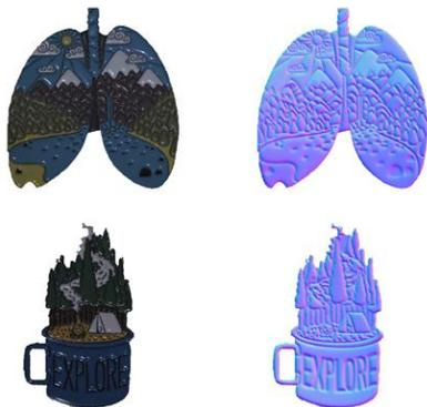
Figure A9: For near-planar objects possessing intricate concave and convex surface details, our LINO UniPS tends to invert the predicted surface normals. The objects are from DiLiGenT-II Wang et al. (2023)
