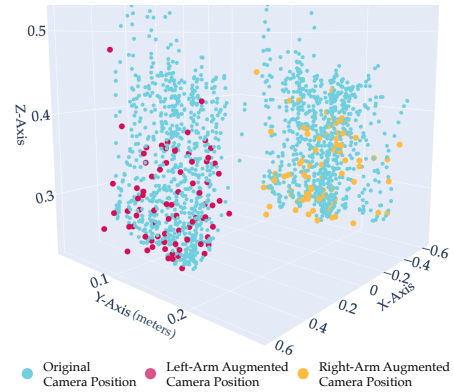
Figure 3: Isometric view of original and augmented camera positions for the real-world Lift Ball task. The augmented camera positions (maroon and yellow dots) provide broader coverage of state-space regions not occupied by the original camera positions (blue dots).
