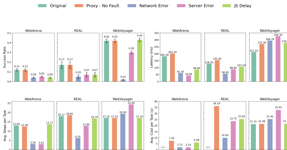
Figure 4: Main Experiments. Mean (a) Success Rate, (b) Latency, (c) Number of LLM calls, (d) Cost per Task for each web failure type in the legend above on each benchmark. All 660 WebArena, 112 REAL, and 643 WebVoyager tasks are considered, and we use GPT-4o as the backbone. 3
