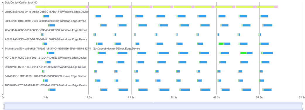
Figure 16: Real-world application on Theta network. Yellow: aggregation server waiting time; pink: aggregation time; green: client training time; blue: client communication.
