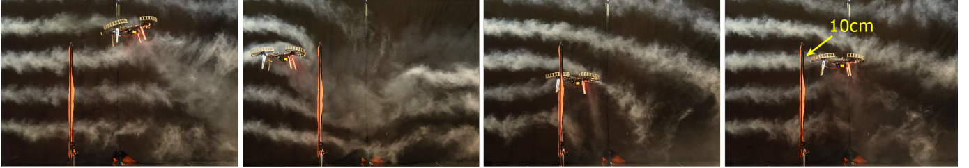
Fig. 3: Agile flight through narrow gates. Neural-Fly was tested in the Caltech Real Weather Wind Tunnel where wind effects can be visualized using smoke machines. The UAV follows an agile trajectory through narrow gates, which are slightly wider than the UAV itself, under challenging wind conditions. These panels show the moment the UAV passed through the gate and the complex interaction between the UAV and the wind.
