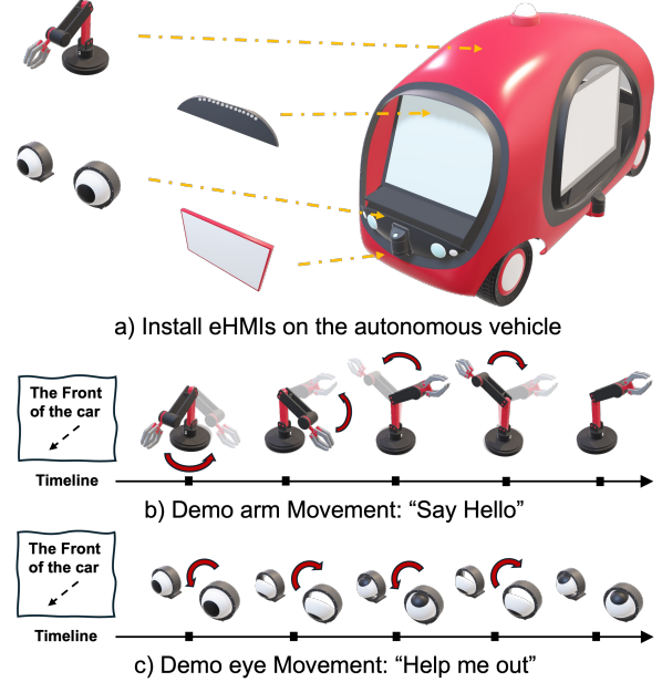
Figure 1: Setup illustration and action demos. a) Four types of eHMIs are installed on the vehicle separately; b) Demo actions of the arm convey the message: “Say Hello”. The shaded action indicates the subsequent status; c) Demo actions of the eye: “Help me out”.
