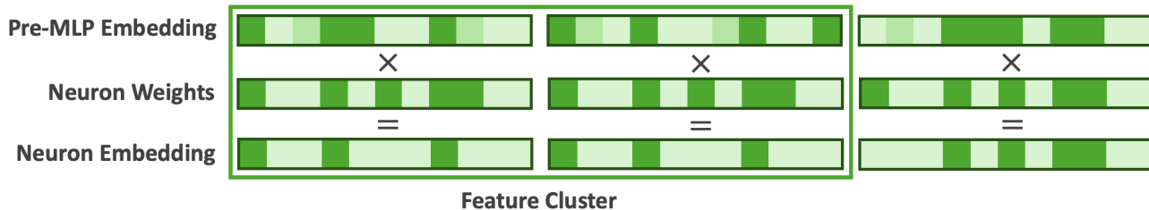
Figure 1. An illustration of the neuron embedding process. We compute the element-wise products of the pre-MLP embedding of the inputs and the neuron input weights to produce the neuron embeddings. These are then clustered based on similarity. The neuron weights select the relevant information from the embedding, such that the neuron embeddings of two different inputs can be brought together or pushed apart.
