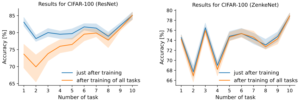
Figure 9: Visualization of mean accuracy (with 95% confidence intervals) of HyperMask for 10 tasks of the CIFAR-100 dataset for two different target network architectures (ResNet-20 and ZenkeNet). The blue lines represent test accuracy calculated after training subsequent models, while the orange lines correspond to test accuracy after finishing training for all CL tasks. Despite the fact that ResNet-20 achieved higher accuracy than ZenkeNet, it suffers from catastrophic forgetting in a more severe way than the second considered architecture.
