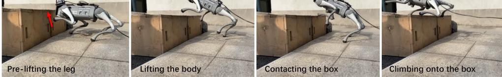
Figure 4: Climbing a wooden box with Lidar
