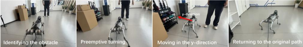
Figure 5: Avoiding a person with Lidar
