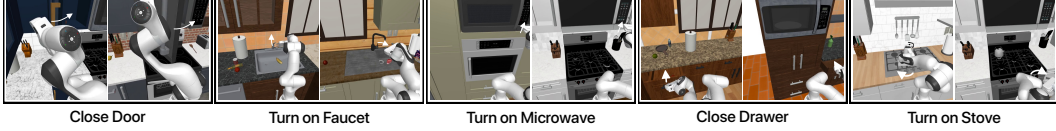
Figure 3: A suite of simulated tasks for benchmarking performance of policy mobilization methods. We pick five single-stage manipulation tasks from the RoboCasa benchmark [20]: (1) Close Door : push or close the microwave or cabinet door using the robot gripper. (2) Turn on Faucet : precisely move the faucet handle to turn on water. (3) Turn on Microwave : push a small button on the microwave. (4) Close Drawer : close an open drawer next to the robot. (5) Turn on Stove : turn a specific knob out of six knobs on the stove. Here, we visualize two successful rollouts for each task. Note that episodes are executed in environments with different layouts and textures.
