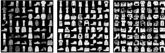
Figure 3. Images generated by the predictor-corrector method with 2000 steps and signal-to-noise ratios of 0.2, 0.5 and 1.0.
