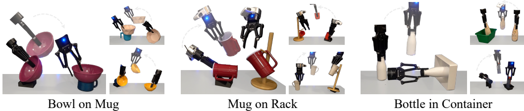
Figure 6: Real Execution Results. Example executions of relational tasks on unseen mugs, bowls, bottles, racks, and containers in the real world. Our framework enables inferring the relative transformation between pairs of unseen objects in arbitrary initial poses from a small handful of unaligned demonstrations of each task.
