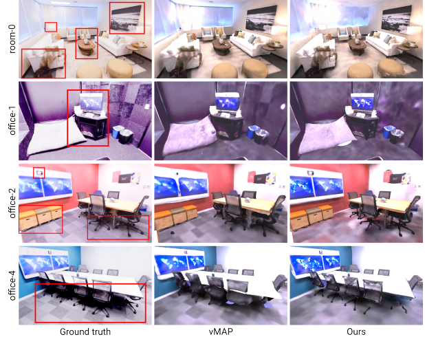
Figure 4. Examples of reconstructions with our method on different Replica scenes, compared to vMAP [33]. Our method recovers object geometry that is more faithful to the actual shapes and with better texture.
