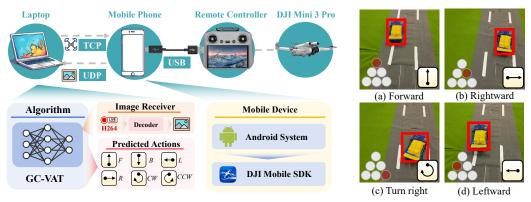
Figure 7: Schematic of the real-world deployment pipeline.
