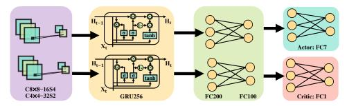
Figure 11: Network structure of Drone Agent.
