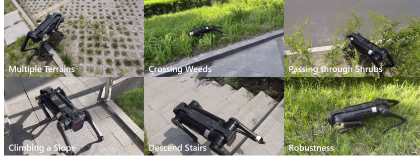
Figure 11: Real-world results for Aliengo robot with different joint failure in different terrains.
