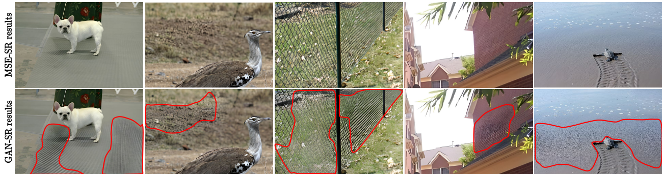
Figure 2. MSE-SR and GAN-SR results of some practical samples. GAN-SR results with artifacts have even worse visual quality than MSE-SR results. The artifacts are complicated with different types and characteristics, and are diverse for different image contents. Regions with red circles are GT of the detection mask.
