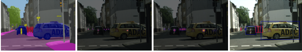
Figure 1: Left : Semantic segmentation prediction. Center left : Poisson point process intensity. Center right : Conditional marked Poisson point process intensity. Right : Bounding box prediction.
