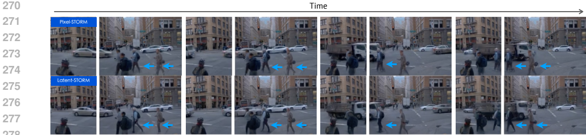
Figure 3: Latent-STORM Examples. Using latent Gaussians and a decoder, Latent-STORM can photorealistically reconstruct human leg movements. Note how the leg angles change over time in Latent-STORM, while they remain static in regular STORM (blue arrows). Please refer to “Human Modeling with Latent-STORM” section in our anonymous page for video comparisons.
