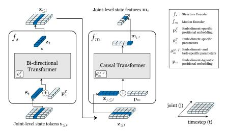
Figure 2: The state encoder f consists of two component transformers. Joint-level state tokens are first encoded by the structure encoder  $f_s$  along the joint axis, where the positional embedding and a part of backbone parameters adapt the model to each embodiment. The features are then passed to the motion encoder  $f_m$ , which computes causal attentions of per-joint features along the temporal axis, where a part of backbone parameters adapt the model both to the embodiment and task.
