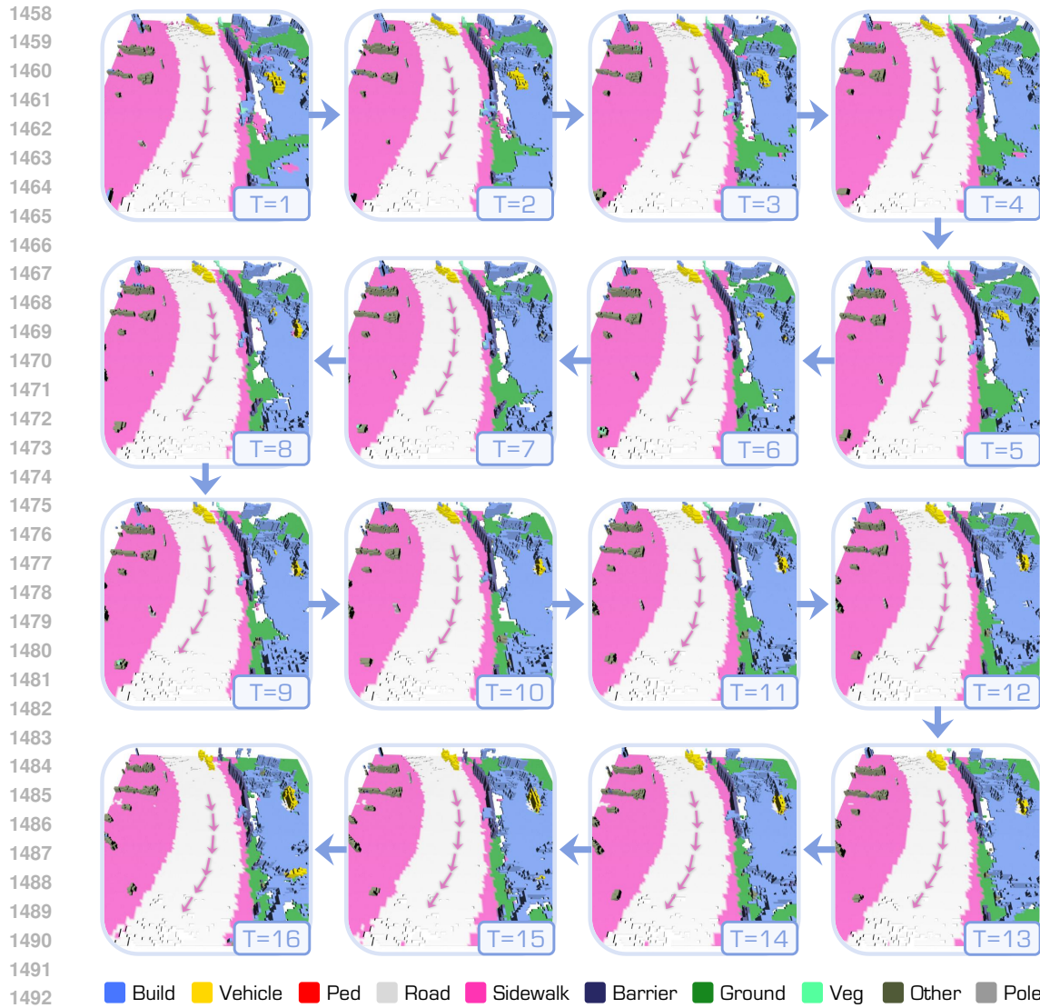
Figure 14: Trajectory-Guided Scene Generation Results. We provide qualitative examples of a total of 16 consecutive frames generated by DynamicCity on the CarlaSC (Wilson et al., 2022) dataset. Best viewed in colors and zoomed-in for additional details.
