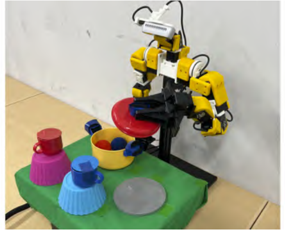
Fig. 2. Experimental environment. A dual-arm robot named Rakuda-2 performed long-horizon tasks involving the manipulation of multiple objects.
