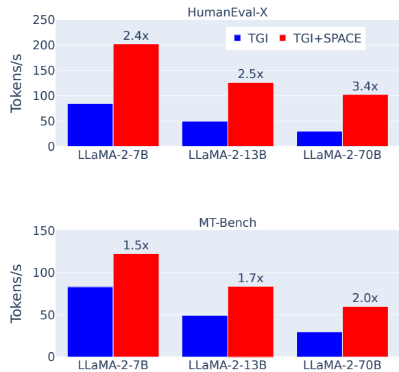
Figure 7: Token generation speed (Tokens/s) and speedup for LLaMA-2 (7B, 13B, 70B) with TGI and SPACE integration on HumanEval-X and MT-Bench datasets under greedy sampling setting. Best viewed in color.
