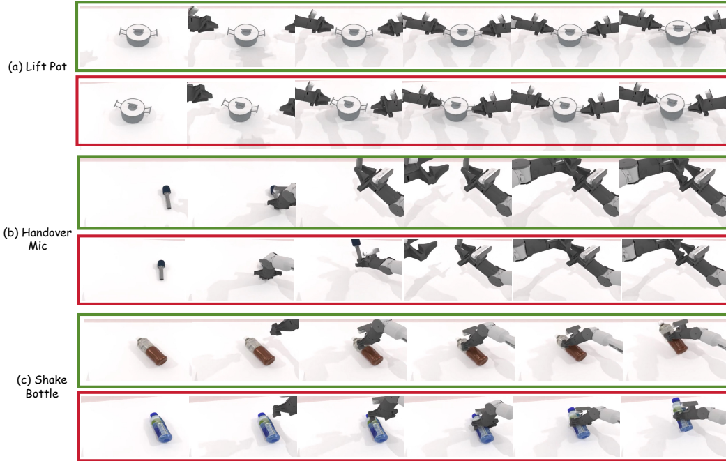
Figure 9: Visualization of policy execution in the Simulation. The green boxes denote the standard egocentric view, the red boxes denote the random novel egocentric view.
