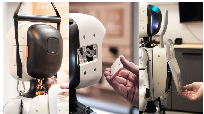
Figure 3: Example product usability features: access panels on the head and backpack including additional compute and networking hardware.
