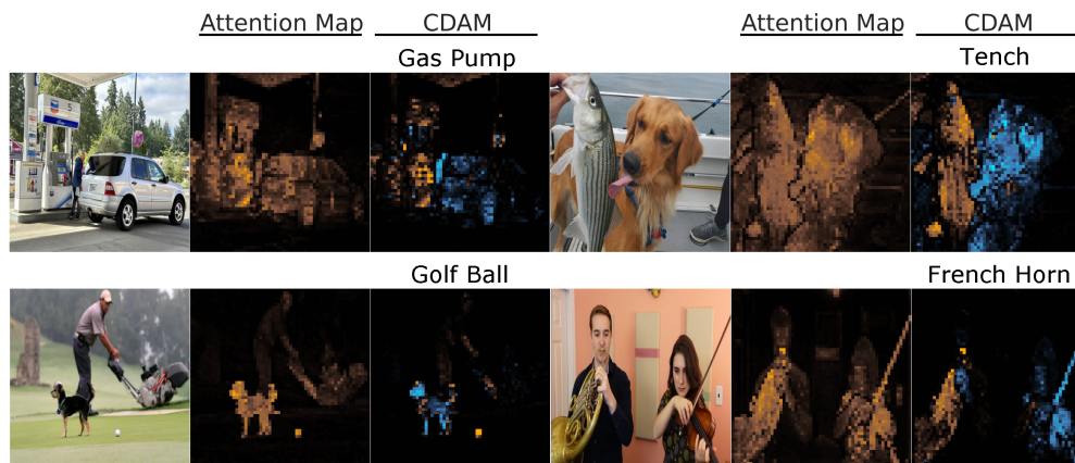
Figure 1: Extending attention maps (AM), the proposed class-discriminative attention maps (CDAM) quantify and visualize input features that are relevant for the target class in Vision Transformers (ViT). We visualize importance scores obtained with CDAM for a linear classifier with ViT-S/8, trained with DINO (Caron et al., 2021). Orange and blue colors correspond to positive and negative values, respectively.
