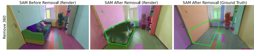
Figure 3: SAM (Kirillov et al. (2023); Ravi et al. (2024)) mask comparison on Remove360. Object removal alters SAM masks, and smaller changes relative to ground-truth masks indicate better removal. These differences are used to compute the similarity score equation 3. Left to right: SAM overlay before removal, after removal, and ground-truth with the object mask (green outline).
