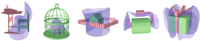
Figure 18: Interaction Bisector Surface (IBS) [ZWK14] is a rich representation between objects in a scene that describes topological and geometric relationships between objects in a scene. IBS is the set of points equidistant from two sets of points sampled on different objects, shown as the blue colored surface above.
