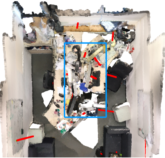
Figure 9: Scene graph pruned by proximity-based KNN. The region of interest is boxed out in blue.
